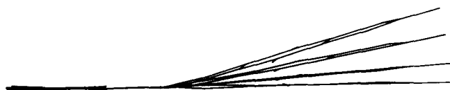
Figure 6 Side view of PBO molecule showing the mode of bending (0, 5, 10, and 15°) used for analysis of the deformation energy
